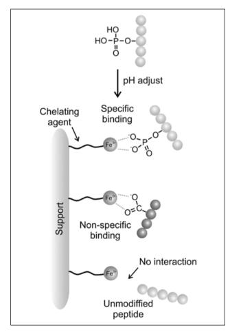
FIGURE 1. ILLUSTRATION DESCRIBING THE OCCURRENCE OF SPECIFIC AND NON-SPECIFIC INTERACTIONS IN AN IMAC COLUMN. SPECIFIC BIDING OCCURS INVOLVING ONLY THE IMMOBILIZED METAL ION AND PHOSPHORILATED PEPTIDES.
