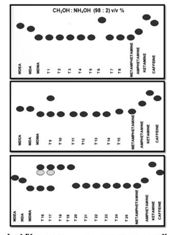
FIGURE 3. TLC DATA FOR THE SEVEN COMMON ECSTASY COMPONENTS TESTED AS WELL AS FOR THE 25 SAMPLES OF APPREHENDED STREET ECSTASY TABLETS USING CH<sub>3</sub>OH:NH<sub>4</sub>OH (98:2) v/v as the eluent. Spots developed by UV are represented by dark black or gray (less intense) ovals.
