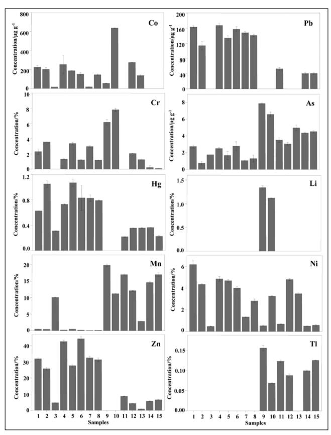
FIGURE 3. CONCENTRATION OF ELEMENTS IN BUTTON CELLS; 1-8: ZN-AIR; 9 AND 10: LI-MNO<sub>2</sub>, 11-15: ZN-MNO<sub>2</sub>. ERROR BARS REPRESENT THE STANDARD DEVIATION FOR THREE BUTTON CELLS (N = 3). BARS NOT SHOWN REFER TO CONCENTRATIONS LOWER THAN THE RESPECTIVE LIMITS OF DETECTION.
