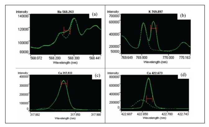
FIGURE 1. EMISSION SPECTRA OF Na (568.263 nm) (a), K (769.897 nm) (b), Ca (317.933 nm) (c) AND Ca (422.673 nm) (d). The SOLID LINE REPRESENTS THE ANALYTE SIGNAL EMISSION AND THE DOTTED LINE THE BACKGROUND SIGNAL.
