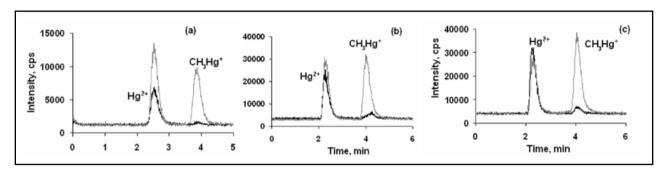
Figure 2. Chromatograms of a standard solution (1.0  $\mu$ g L<sup>-1</sup> Hg) and mushroom sample. (a) US assisted extraction; (b) MW assisted extraction; (c) conventional extraction. Gray line: standard solutions; black line: mushroom sample.
