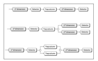
FIGURE 3. DIFFERENT CONFIGURATIONS EMPLOYED FOR THE SEPARATION OF PROTEINS USING ON-LINE TWO-DIMENSIONAL CHROMATOGRAPHIC SYSTEMS. THE USE OF MULTIPLE TRAP COLUMNS OR MULTIPLE COLUMNS FOR THE SEPARATION IN THE SECOND DIMENSION ALLOWS INCREASE IN THE ANALYTICAL FREQUENCY OR A HIGHER SAMPLE FRACTIONATION DURING THE SEPARATION IN THE FIRST DIMENSION.
