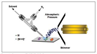
Figure 2. Schematic of TLC/EASI-MS. Supersonic spray produces a bypolar stream of very minute charged droplets (blue spray) that bombard the TLC silica surface causing desorption and ionization of the analyte molecules that rest on the target spot (green dots). Analytes are ionized often as  $[M=H]^+$  or  $[M-H]^+$ , or both. EASI is assisted only by compressed nitrogen or air, and causes no oxidation, electrical, discharge, or heating interferences.
