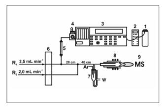
Figure 1. Squematic diagram of the LC-CVG-ICP-MS system. 1: mobile phase (L-cysteine); 2: vacuum degasser; 3: LC pump; 4: injector; 5: column (Si- $C_{18}$ ); 6: peristaltic pump; 7: gas-liquid separator (L = 10 cm; i.d. = 15 mm); 8: ICP; 9: mass spectrometer;  $R_1$ : HCL (1.0 mol  $L^{-1}$ );  $R_2$ : NaBH, (0.25% m/v).
