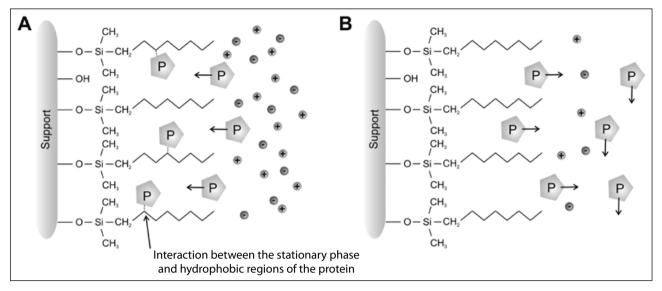
FIGURE 2. SCHEMATIC REPRESENTATION FOR THE SEPARATION OF HYDROPHOBIC PROTEINS THROUGH HIC. (A) IN THE PRESENCE OF HIGH CONCENTRATION OF COSMOTROPIC IONS, AND (B) AFTER REDUCING THE SALT CONCENTRATION, PROMOTING THE GRADUAL ELUTION OF PROTEINS.
