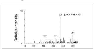
FIGURE 6. EASI-MS COLLECTED DIRECTLY ON THE SURFACE OF THE SINGLE TLC SPOT FOR TABLET T18.
