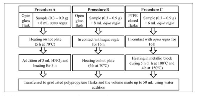
FIGURE 2. SUMMARY OF PROCEDURES INVESTIGATED FOR BUTTON CELLS DECOMPOSITION (ZN-AIR BUTTON CELLS WERE USED).
